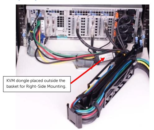
Figure 5: Right-Side Mounted CMA Installation
